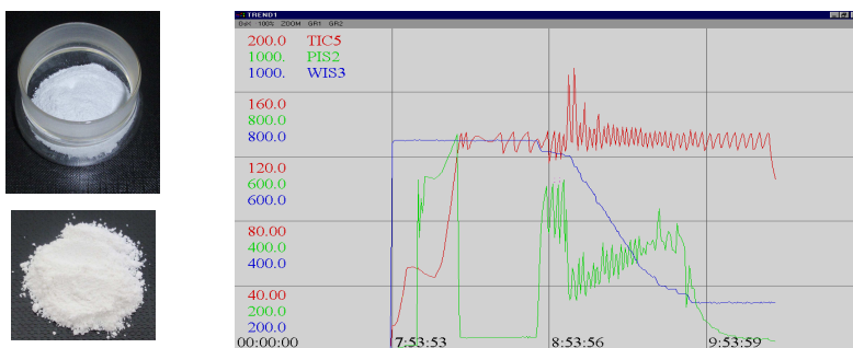
Fig. 1. Activity Control Test of MEO-DMC catalyst during propoxylation of polypropylene glycol 450, at 27 ppm concentration, where: blue line means weight of alkylene oxides in feeding vessel, red line denotes temperature, green line sets pressure during synthesis.
